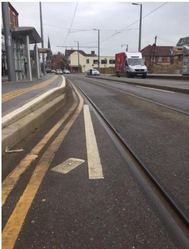
*Like many others John didn't realise the danger by the tram stop. The pavement is raised and there is a very narrow space between it and the tram track. The double yellow lines create a further hazard.*
